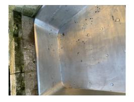
EXAMPLE OF FLUX DAMAGED BATH AFTER INSTALLATION
